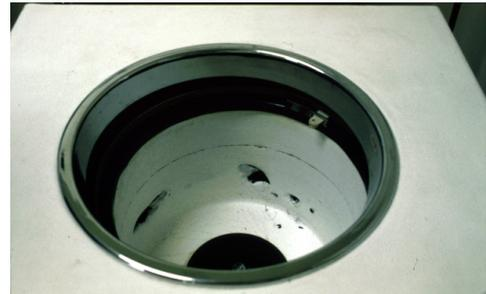
The bucket came off from the running rotor at 40,000 rpm and crashed onto the chamber wall at a velocity of over 1,600 km/h. Relative Centrifugal Field is 193,000 g.
