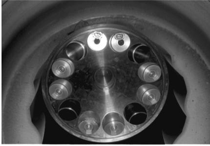
The driving unit was damaged, while the titanium rotor installed to the spindle was intact.
