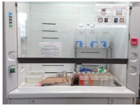
Draft Chamber Use organic solvent under the draft chamber
