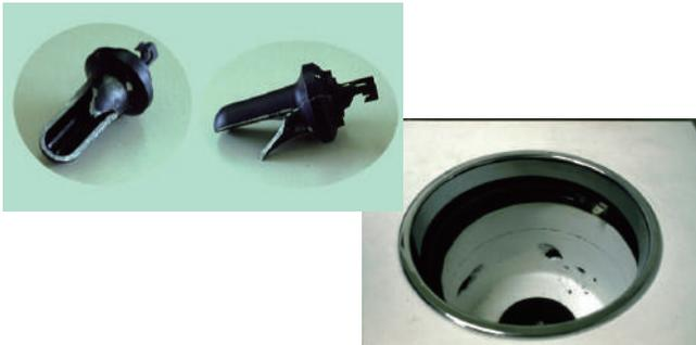
The bucket came off from the running rotor at 40,000 rpm and crashed onto the chamber wall at a velocity of over 1,600 km/h. Relative Centrifugal Field is 193,000 g.
