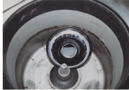
The rotor came off from the spindle and rolled around in the chamber. The rotor and spindle were severely damaged.
