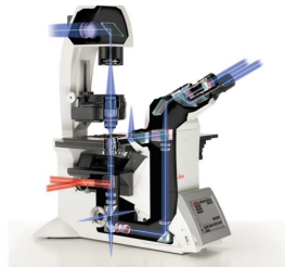
Figure 8: An upright microscope features the objective above and the condenser below the specimen (left). On an inverted microscope this set-up is turned around (right).
