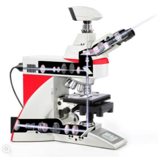
Figure 8: An upright microscope features the objective above and the condenser below the specimen (left). On an inverted microscope this set-up is turned around (right).
